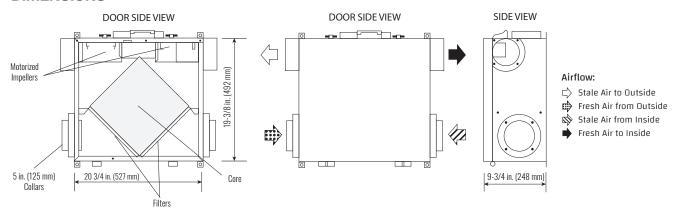
NOTE: Front clearance of 25 in. (635 mm) is recommended for servicing unit. All ducts use 5 in. (125 mm) round collars. MERV 13 upgrade: 485463 Weight: 34 lbs (15.5 kg) • Shipping weight: 36 lbs (16 kg)
