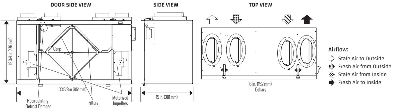
NOTE: Front clearance of 25 in. (635 mm) is recommended for servicing unit. All ducts use 6 in. (152 mm) oval collars, balancing dampers are located on all collars. MERV 13 upgrade: 485467. Weight: 57 lbs (25.8 kg) • Shipping weight: 67 lbs (30 kg)
