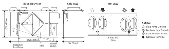
NOTE: Front clearance of 25 in. (635 mm) is recommended for servicing unit. All ducts use 6 in. (152 mm) oval collars, balancing dampers are located on all collars. MERV 13 upgrade: 485467. Weight: 57 lbs (25.8 kg) • Shipping weight: 67 lbs (30 kg)
